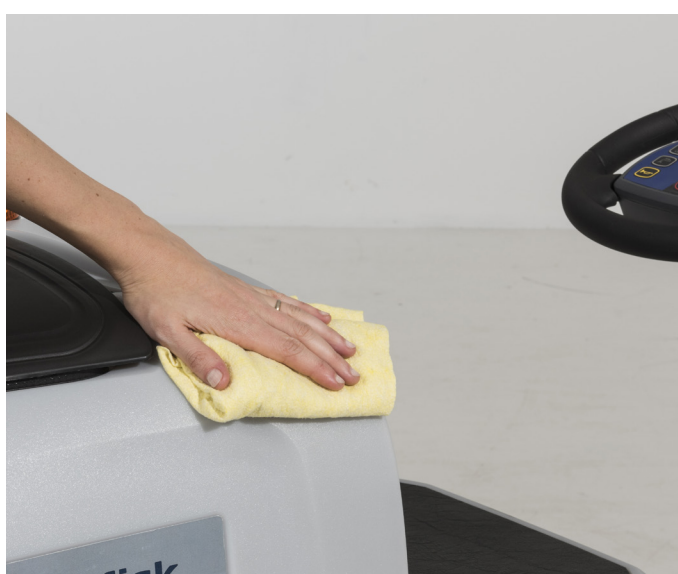
15. Clean the machine using a damp cloth and where needed use a neutral cleaning product.
