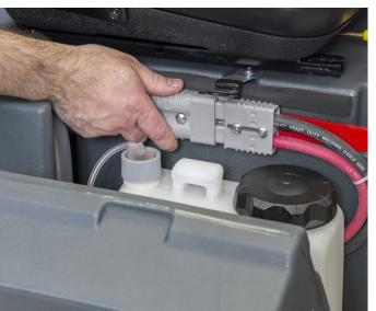
3. Check battery cables are well connected together
