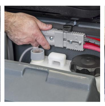
3 Check battery cables are well connected together.
