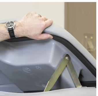
Recovery tank seal cover must 4 correctly installed and in good condition.
