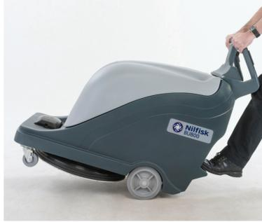
3. Tilt the machine in order to have access to pad retainer
