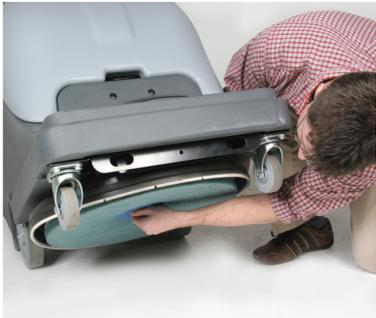
6. Retighten the pad retainer as tight as possible
