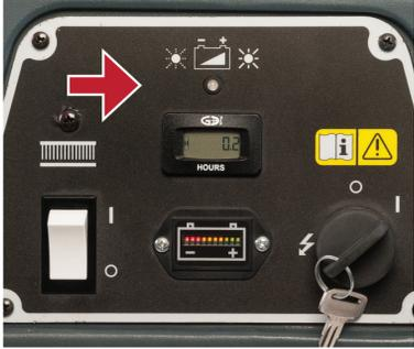
1. If the battery is on charge, check if the battery charger indicator shows a green light (it means the battery is fully charged)
