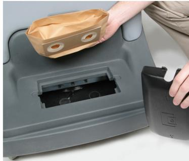
8. Remove the cover of passive dust collector and replace dust bag if it is full or torn
