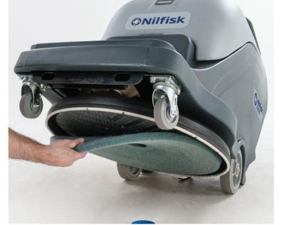
5. Remove the pad and check the status. If needed, change it. Be sure to use correct burnishing pad depending on floor type and application
