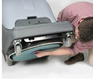
4. Rotate the retainer and remove it from the machine.
