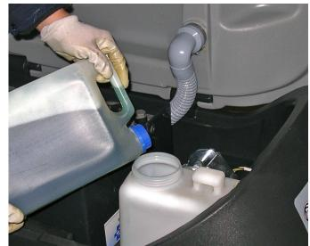
3. Fill the EcoFlex<sup>™</sup> tank with a detergent suitable for the work to be performed (highly concentrated detergent).
