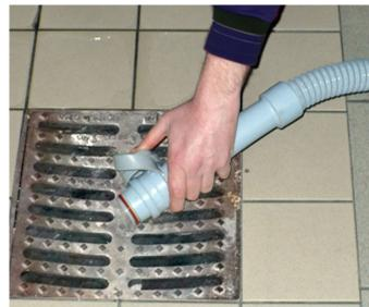
12. **At the end of the work.** Empty the recovery tank with the hose. Then empty the solution tank with the trasparent hose
