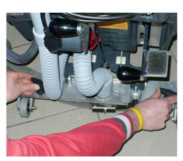
4. Install the squeegee and fasten it with the handwheels, then connect the vacuum hose to the squeegee.
