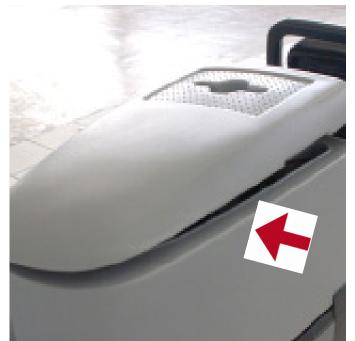
Close the recovery tank cover properly and/or verify the gasket wear.
