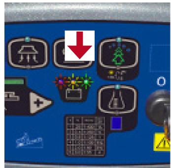
2 Check if there isn't any brush motor 3 overload i.e. 3 battery Ledsflash simultaneously.
