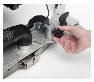
3. If the squeegee is not connected to the machine: install and fasten it with the handwheels, then connect to the suction hose.
