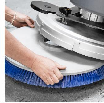
**1** Check if the brush is correctly installed and not worn out.
