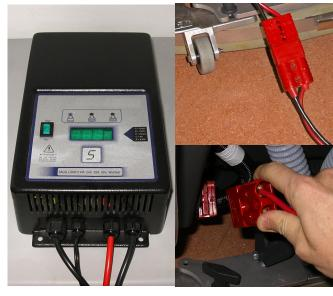
1a. Switch off charger by unplug charger cable from red battery plug. Reconnect the red battery plug to the machine.
